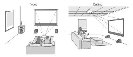
Ideally, keep the projector level and place it at a height so its lens is centered between the top and bottom of the screen. If this is not possible, use the lens shift dials to reposition the image. As a rule of thumb, you can use lens shift to move the image up or down by nearly its full height, and left or right by about one-half its width (for details, see page 22).
